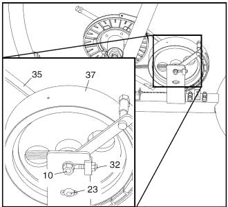
Next, loosen, but do not remove, the M8 x 20mm Bolt (23). Loosen the two M8 Nylon Locknuts (10), one on each side of the Flywheel (37). Tighten the M6 Nylon Locknuts (32), one on each side of the Flywheel, until the Belt (35) is properly tightened. Then, tighten the M8 Nylon Locknuts (10) and the M8 x 20mm Bolt (23). Finally, reattach the side shields, the upright covers, and the pedals.
